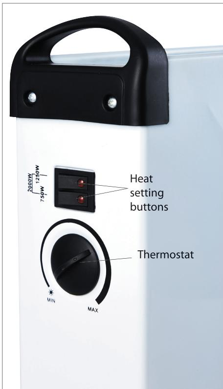
The electric radiator is equipped with an automatic circuit breaker which is activated in the event of overheating. If this circuit breaker is activated, you should switch off both heat setting buttons and pull the plug out of the socket. Then allow the electric radiator to cool off and remove anything that may be blocking the flow of air before turning the electric radiator back on. If the automatic circuit breaker is activated repeatedly, the electric radiator needs to be serviced.
