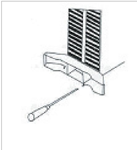
Each foot requires two screws. Once the feet are attached, you should check that the electric radiator stands steady and stable.
